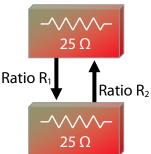
The 1:1 measurement ratio can be easily calibrated and verified by interchange measurement tests using two stable standard resistors of same nominal values, as illustrated by the block diagram to the right. Bridge 1:1 measurement ratio error  $e_i$  (in ppm) is calculated using the following formula:
